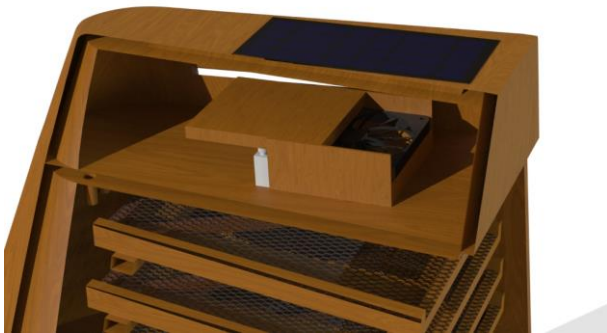
Figure 7: View of the solar panel and fan
